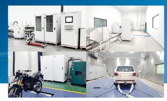
The Gasboard-9802 full-flow dilution constant volume sampling (CVS) system is designed for the measurement of diluted emissions from vehicles and engines. It has a complete and technologically advanced hardware configuration and software platform. When used in conjunction with a high-precision gas and particle online analyzer, it meets cold-start emissions test requirements under normal laboratory conditions for major mobile source emission standards, including the upcoming Euro 7 standard.
